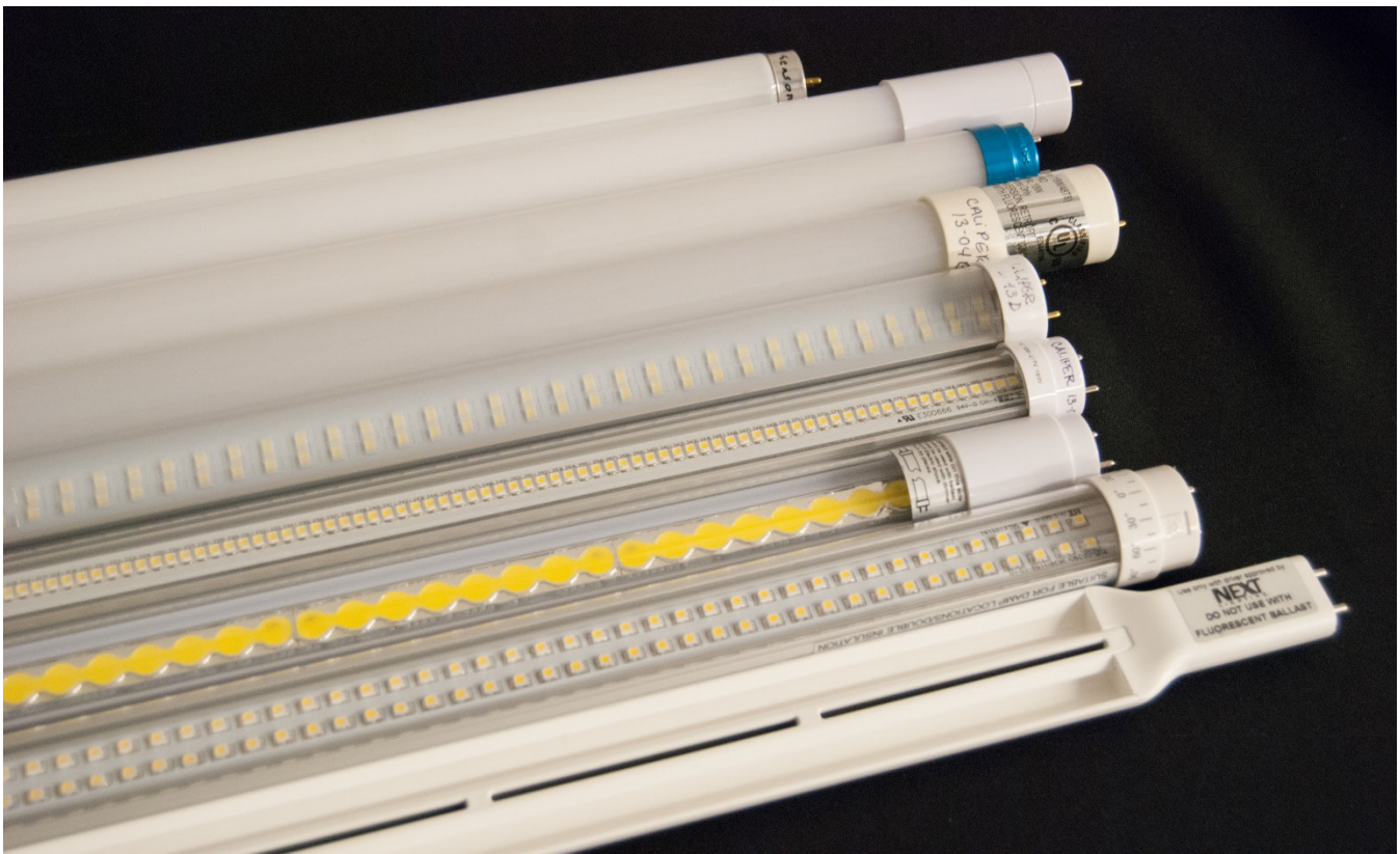
Figure 1. A subset of the Series 21 linear LED lamp (and fluorescent benchmark, top), illustrating the range of product designs. The lamps were staggered when the photo was taken; they are all approximately the same length.
